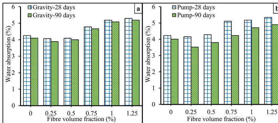
Fig. 10. The variation in water absorption of PAFRC specimens for (a) gravity method; (b) pumping method.
