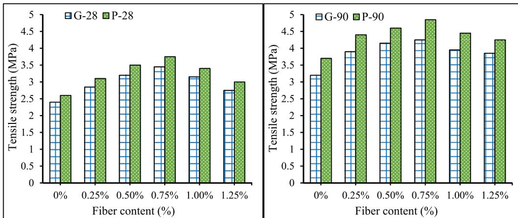
Fig. 9. Tensile strength of PAFRC mixes with different fiber volume fractions.
