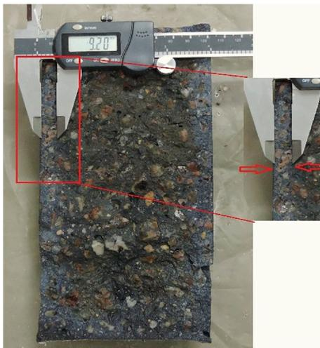
Fig. 6. The depth of chloride penetration depth measurement.
