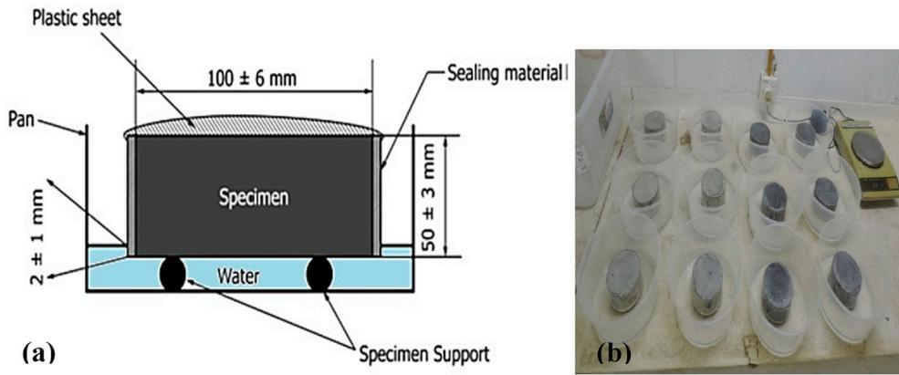
Fig. 5. (a) The procedure of sorptivity test; (b) concrete disk specimens used.
