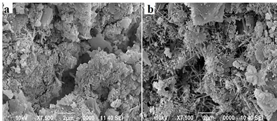
Fig. 8. SEM images of (a) OPC and (b) POFA grouts used in PAC at 90 days.
