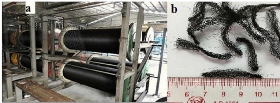
Fig. 2. (a) The yarn used in carpet manufacturing; (b) Fabricated waste carpet fibers used.
