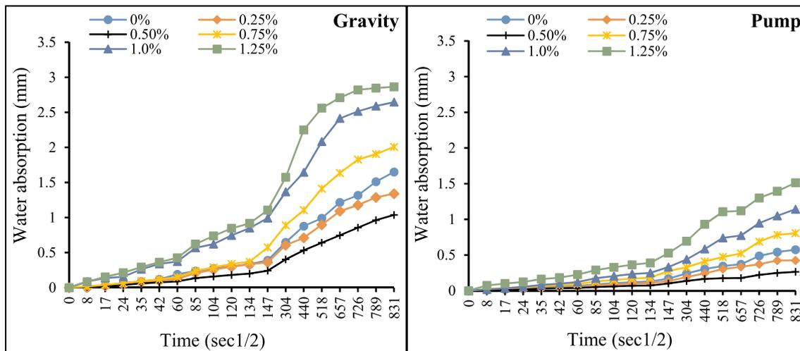
Fig. 11. Water absorption vs. square root of time for gravity and pumping methods PAFRC specimens.
