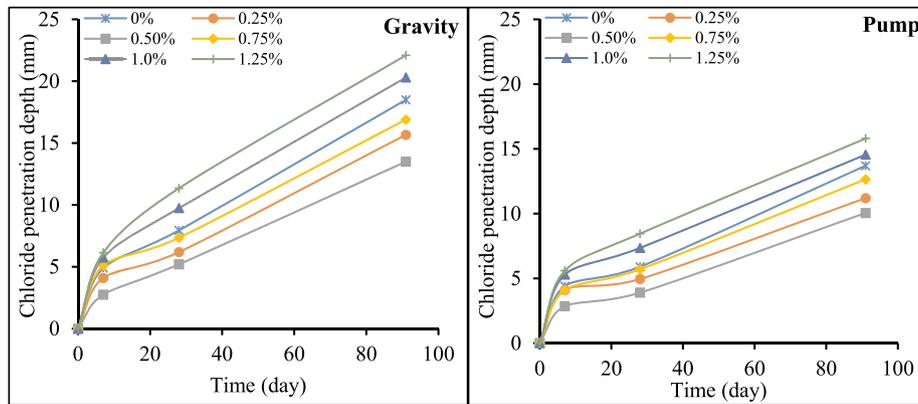
Fig. 12. Effects of carpet fibers on the chloride penetration depth for (a) gravity method and (b) pumping PAFRC specimens.
