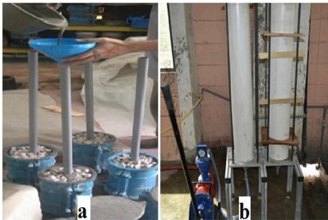
Fig. 3. Grouting methods of PAFRC: a) Gravity; b) Pumping.
