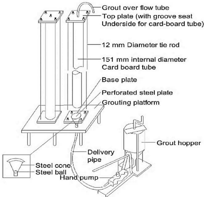
Fig. 4. Schematic process of grouting by pumping method.
