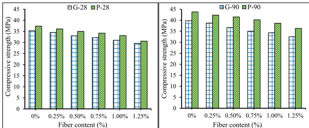
Fig. 7. Compressive strength of PAFRC mixes vs. fiber content.
