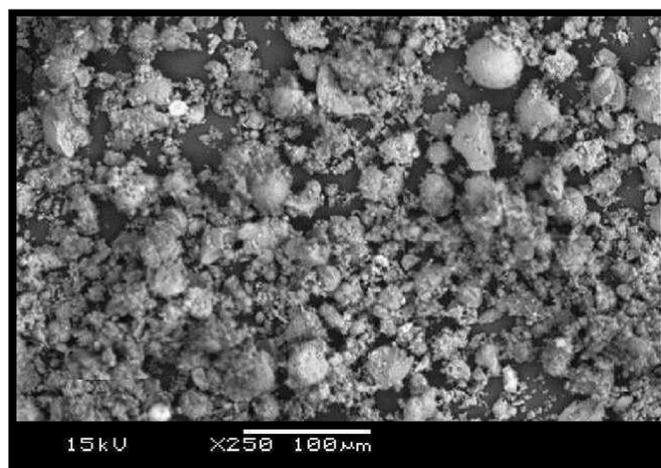
Fig. 1. Scanning electron micrograph of POFA.
