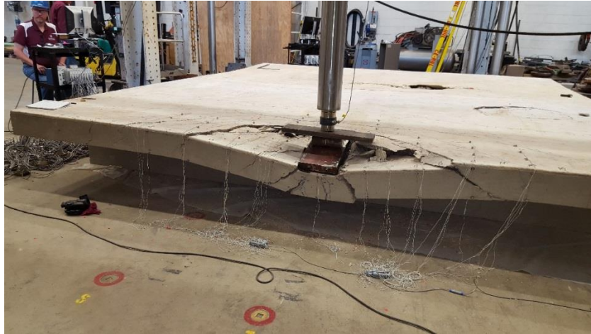
Figure 170. Damage at End of LP3 Test
