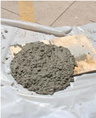
Figure 119. Significant Slump of Fresh Mix without Steel Fibers
