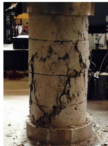
Figure 58. A Failed SFRC Specimen after the Compression Test
