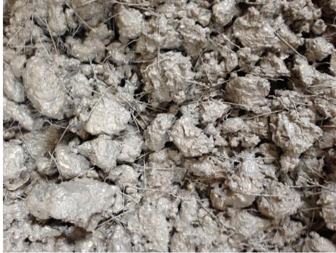
(a) Uniformly Distributed SFRC (H05)
