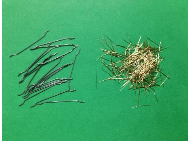
Figure 52. Hooked Steel Fiber (Left) and Straight Steel Fiber (Right)
