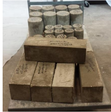
Figure 122. Casts for ASTM Materials Tests on Way to Curing Room
