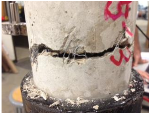
(a) Cracking of SFRC
