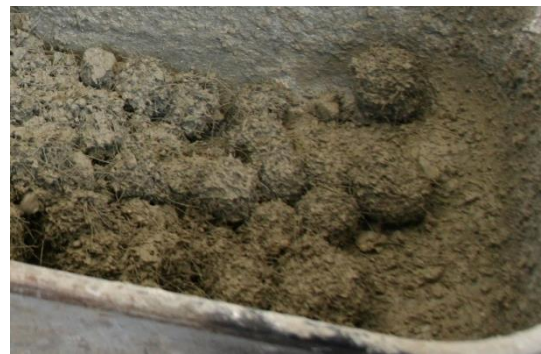
Figure 117. Significant Clumping in SFRC
