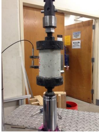
Figure 57. Tension Specimen Setup
