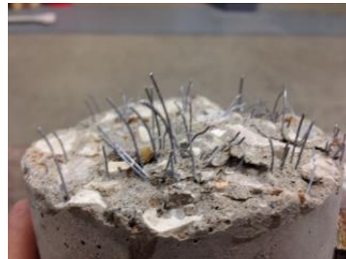
(b) Pulled Out Fibers
