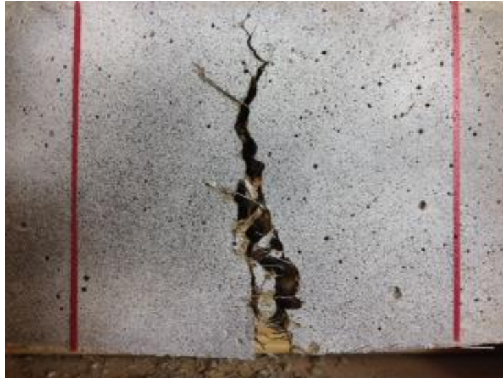
Figure 82. A Failed Flexural Specimen
