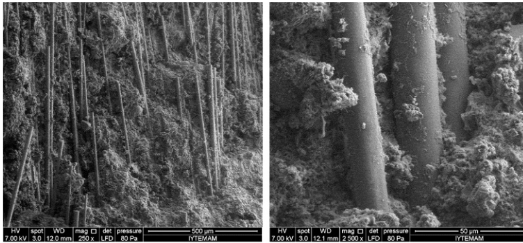
Fig. 8.9 SEM images of basalt fiber-reinforced concrete.
