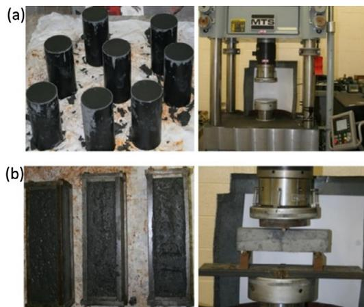
Fig. 2. (a) HPFRC specimens and the experimental setup for compressive stiffness test. (b) HPFRC specimens and the experimental setup for bending stiffness test.
