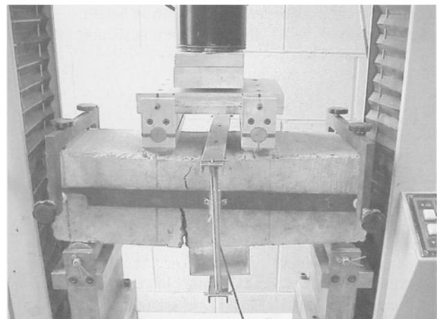
Fig. 2 - Set-up for flexural toughness test.
