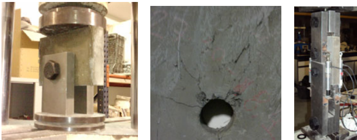
Fig. 5. From left to right: Bearing strength test set up, bearing failure mode and connection test
