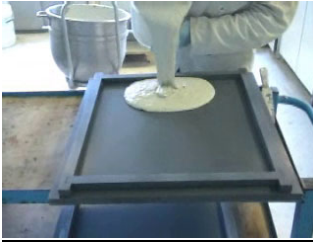
Fig. 1. Self-placing properties. The plates are sawn in the direction of casting after demolding
