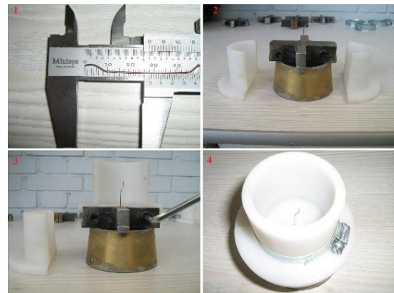
Fig. 7. Fiber installation in pull-out specimen mold
