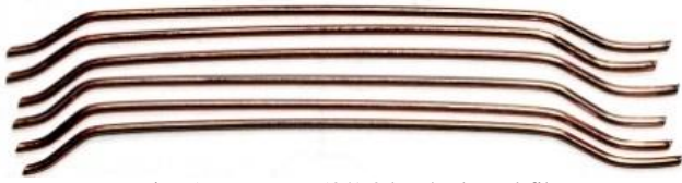
Fig. 5. Durocem 50/1.0 hooked steel fiber
