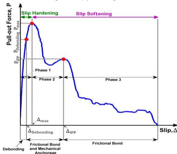
Fig. 2. General pull-out force vs. slip behavior of hooked steel fiber from cementitious matrix [12,13]
