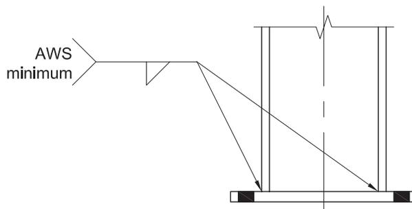
Fig. 4-15. Typical gravity column base plate weld.
