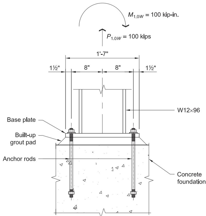
Fig. 4-35. Base configuration and dimensions used in Example 4.7-13.
