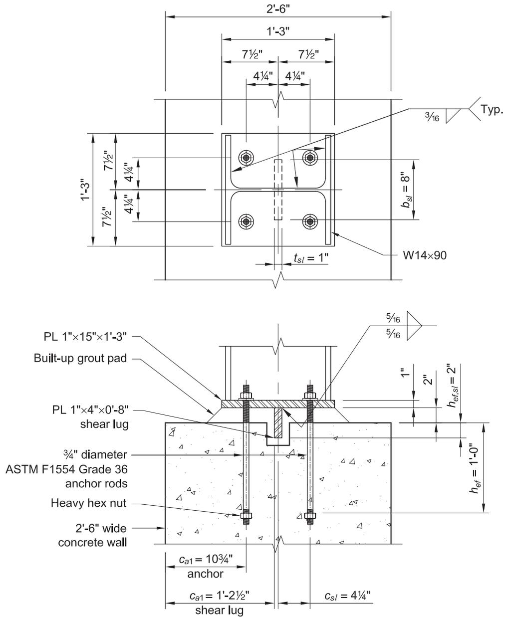
Fig. 4-26. Base connection as detailed in Example 4.7-5.
