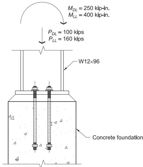
Fig. 4-32. Base detail section as used in Example 4.7-10.
