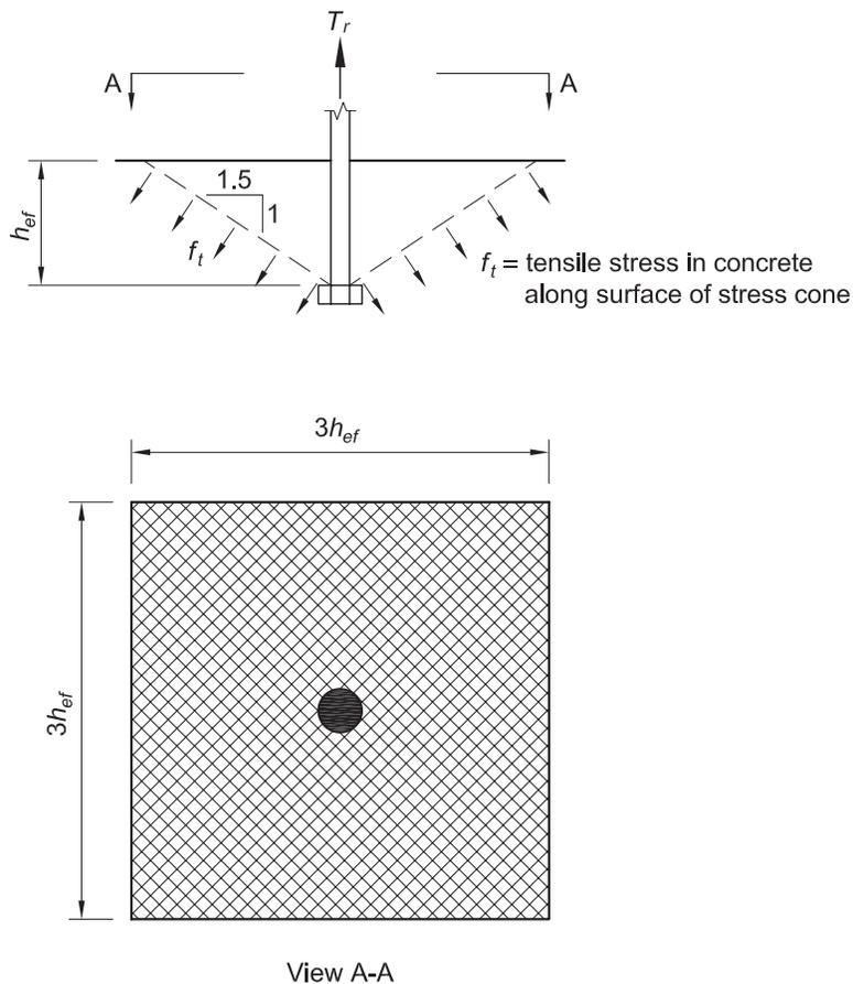
Fig. 4-2. Full breakout cone in tension per ACI 318.
