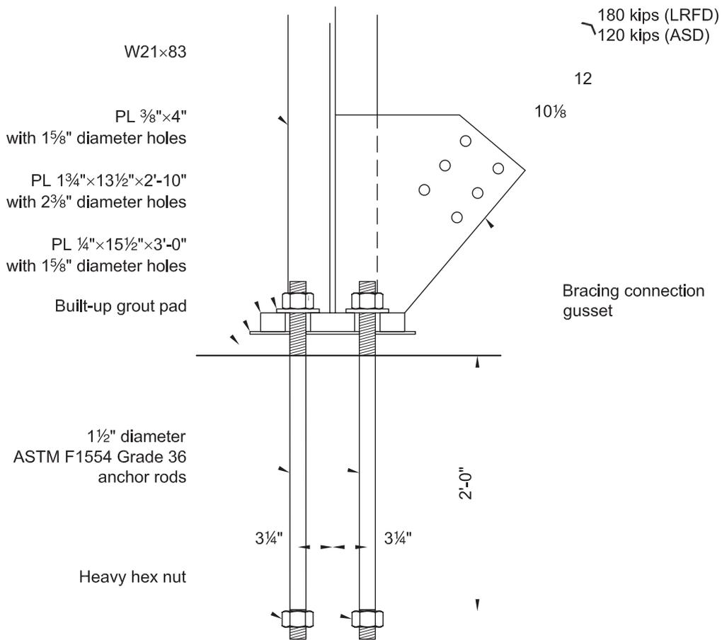
Fig. 4-28. Base connection as detailed in Example 4.7-7.
