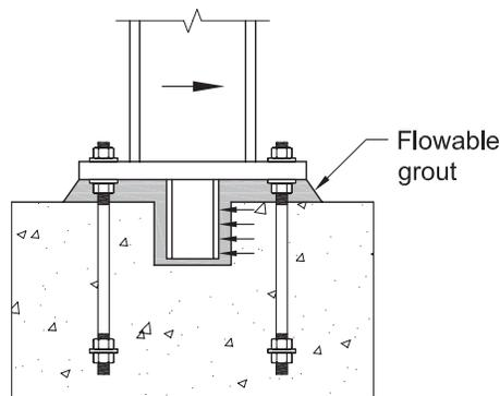
Fig. 3-3. Shear lug to resist large shear forces.
