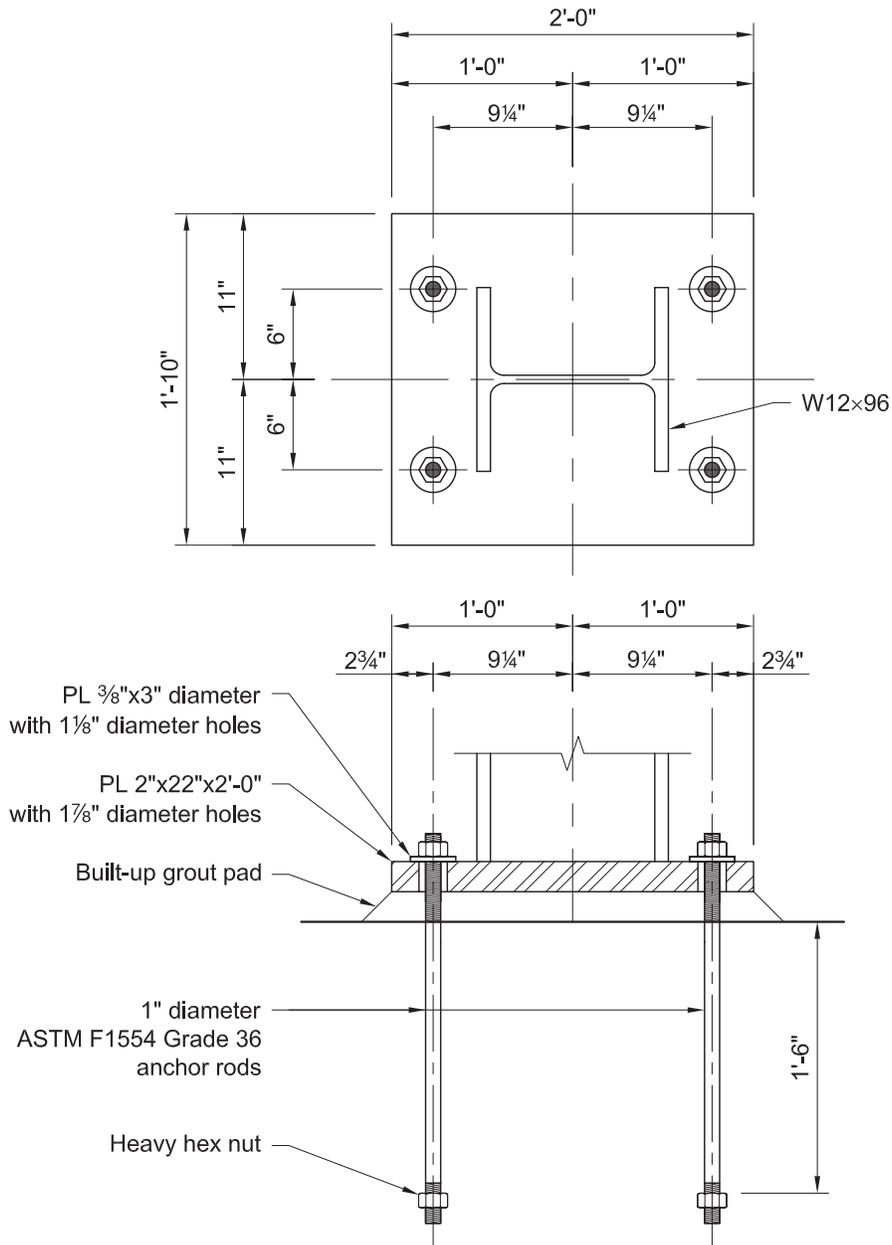
Fig. 4-33. Base connection as detailed in Example 4.7-11.
