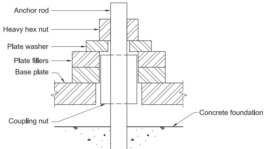
Fig. 4-18. Coupling nut detail for extending anchor rods.
