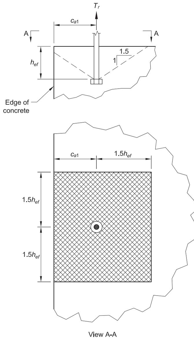
Fig. 4-3. Breakout cone in tension near an edge.
