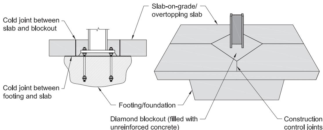
Fig. 3-5. Breakout connections resulting in shallow embedment of base plate connections.
