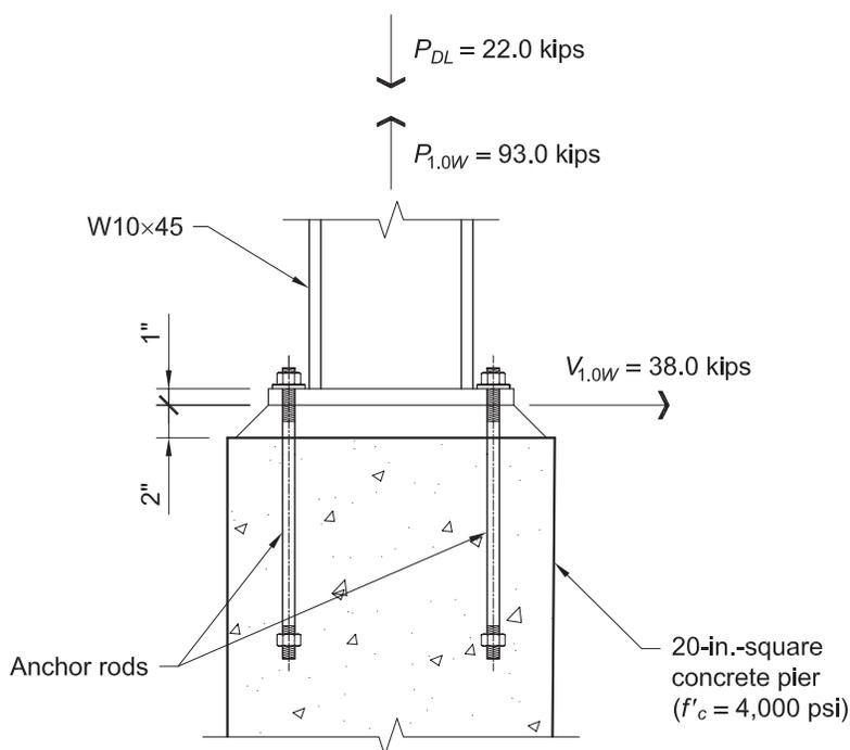
Fig. 4-27. Applied loading and base connection configuration used in Example 4.7-6.
