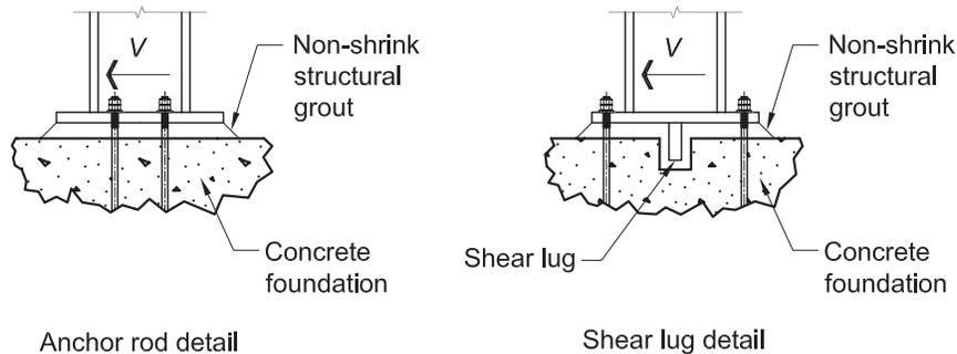
Fig. 4-5. Transfer of base shear.
