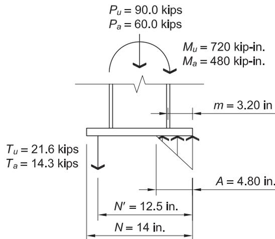
Fig. B-4. Design example with large eccentricity.
