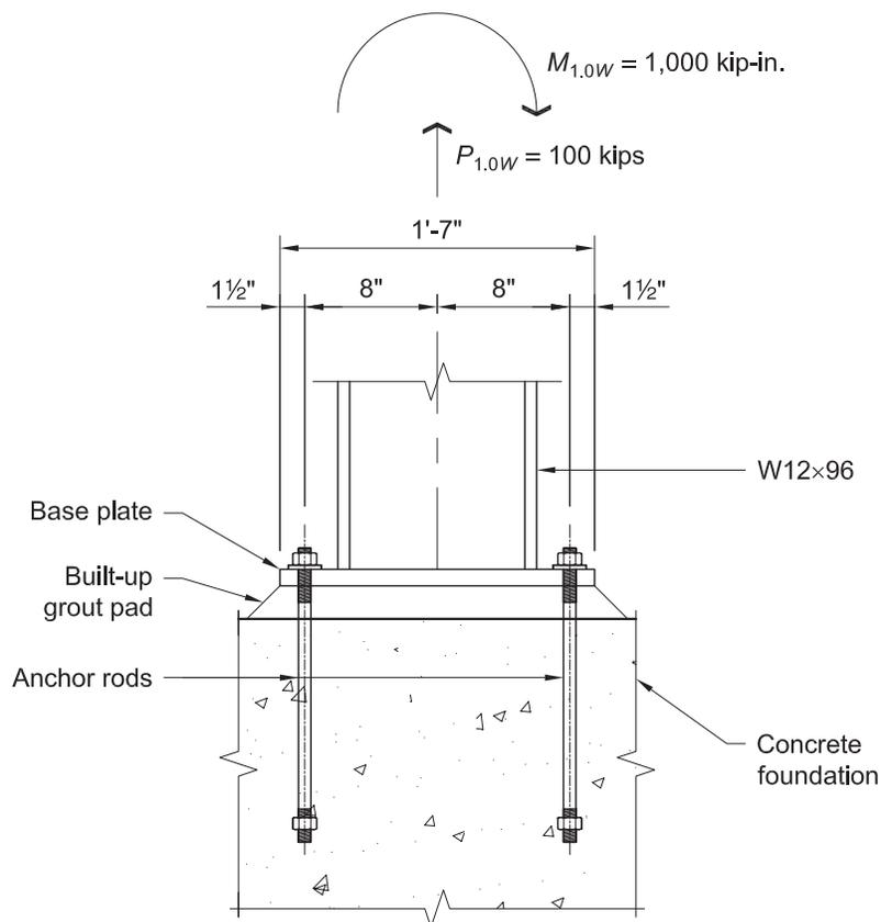
Fig. 4-34. Base connection configuration as detailed in Example 4.7-12.
