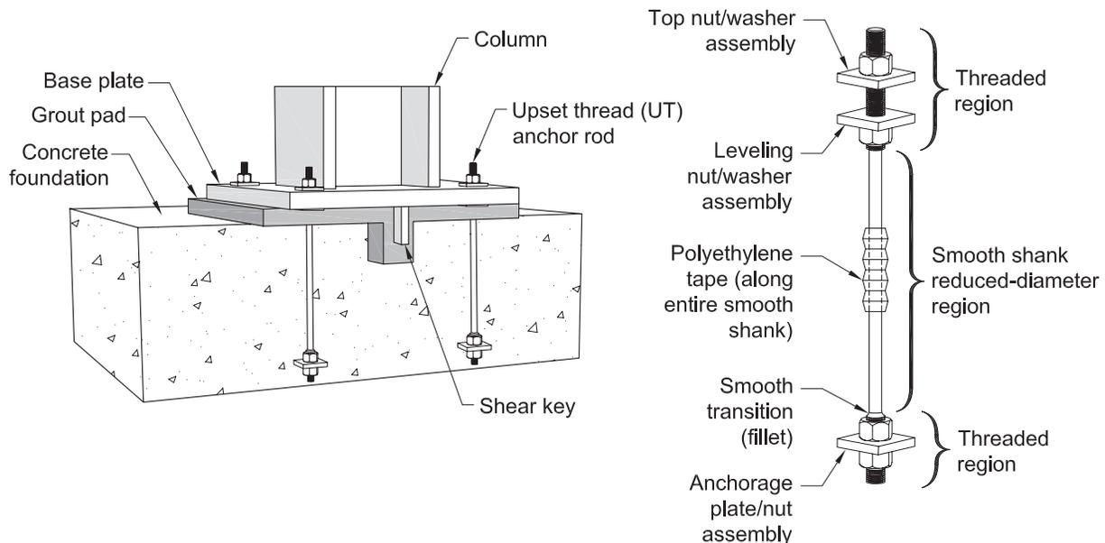
Fig. 6-1. Upset thread detail for weak-base seismic design.
