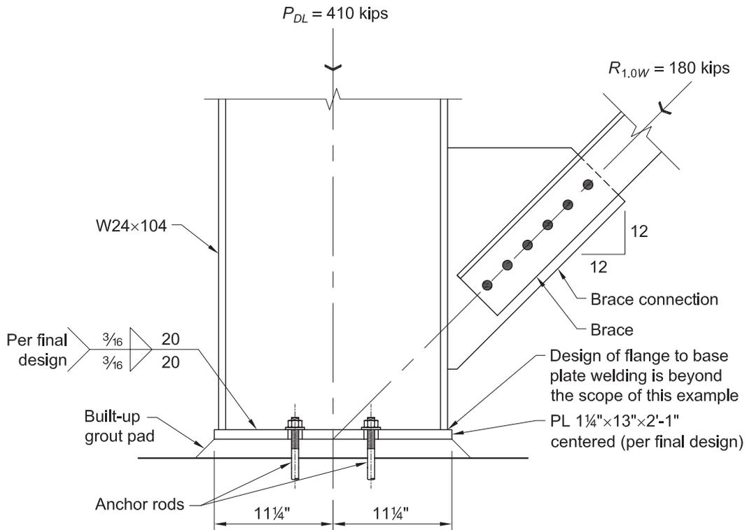
Fig. 4-30. Base connection elevation view detailed in Example 4.7-8.
