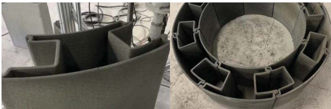
Figure 6-61 Concrete components fabricated using 3D printing
