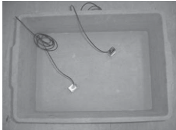
Figure 8-20 Placement of the transducers before casting
