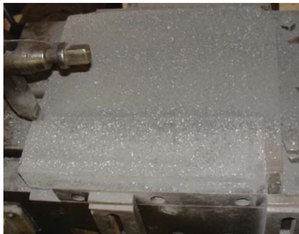
Figure 6-22 Extruded products can easily be machined (milling)
