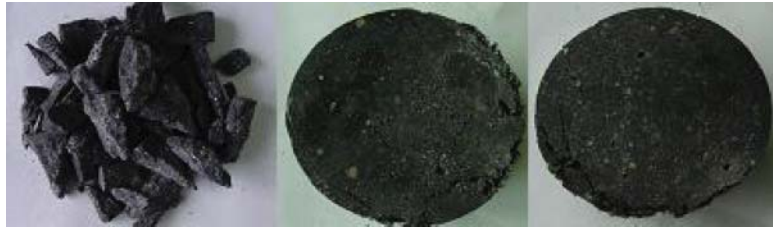
Figure 6-34 Influence of fiber on UHSC impact resistance
