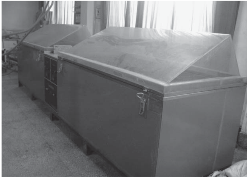
Figure 5-77 Seawater tank for marine environmental simulation test
