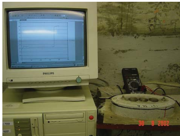
Figure 5-47 Elliptical ring test for constrained shrinkage: (a) sketch; and (b) photo of equipment
