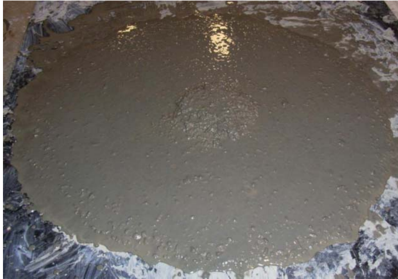
Figure 6-43 Slump flow of SCC that suffers from lack of cohesiveness
